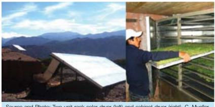
Source and Photo: Two unit rack solar dryer (left) and cabinet dryer (right), C. Mueller, Fundación EcoAndina
